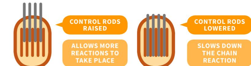
Control rods, commonly made of boron or cadmium, can be lowered into the reactor. They slow the reaction by absorbing neutrons, meaning there are less available to trigger fission.
