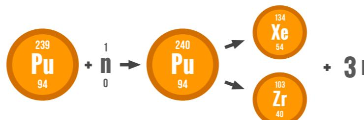
Plutonium-239 is generated by neutron collision with uranium-238, and is also fissionable, creating around one third of a nuclear reactor's energy.
