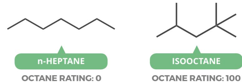
Knocking occurs when fuel's combustion doesn't occur in sync with the engine cycle. This causes lower engine efficiency and engine damage. Octane ratings gauge how well fuel avoids this problem, with higher values indicating less knocking. Isooctane (100) and n-heptane (0) are used as references.
